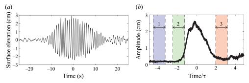
Figure 2. (*a*) Example surface elevation of a single wave group (case *D*), measured by a wave probe at the SPIV measurement location. (*b*) Ensemble-average group amplitude envelope as a function of time for case *A*. The time intervals for SPIV measurement are shaded.
