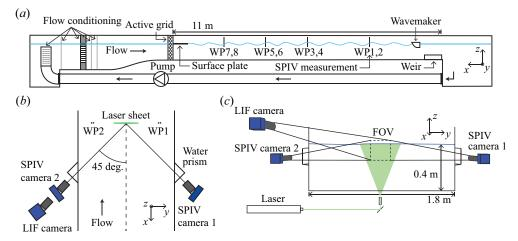
Figure 1. Experimental set-up: (a) side view of water channel (WP, wave probe) with flow from left to right, (b) top view of measurement region, (c) longitudinal view. FOV, field of view.
