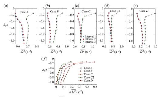
Figure 4. (*a–e*) Cross-plane enstrophy  $\overline{\Omega^2}(z)$  for cases and time intervals as indicated. (*f*) Measured increase of  $\overline{\Omega^2}(z)$  from interval 2 to 3 for all cases.
