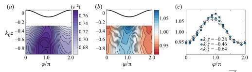
Figure 3. Ensemble-averaged cross-plane enstrophy in regular waves (case C3). (a)  $\Omega^2(z, \varphi)$ ; (b)  $\overline{\Omega^2}(z, \varphi)/\langle \overline{\Omega^2} \rangle_{\varphi}(z)$  (Eulerian reference frame); (c)  $\overline{\Omega^2}(\zeta, \varphi)/\langle \overline{\Omega^2} \rangle_{\varphi}(\zeta)$  (surface-following reference frame), for values of  $k_0 \zeta = k_0 (z - \bar{\eta}(\varphi))$  given in the legend.
