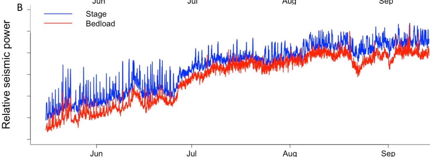
Figure 3 Time series from the hydrological gauging station and geophones at location A and the geophones at location B at Leverett glacier, showing relative stage and bedload transport over summer 2022. The blue line, interpreted as relative stage, represents the sum of the 0 – 20 Hz frequency range, while the red line, interpreted as relative bedload, represents the sum of the 20 – 50 Hz frequency range.
