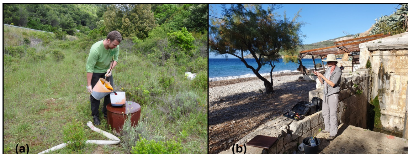
Figure 6. Activities performed in the scope of research: (a) tracer test (dye injection); (b) water sampling at Kamenice spring.
