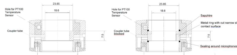
Standard Brüel & Kjær plane wave coupler (left) modified to prototype coupler for Infra-AUV measurements (right)
