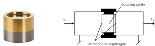
LS microphone Brüel & Kjær Type 4160 and sketch of measurement configuration
