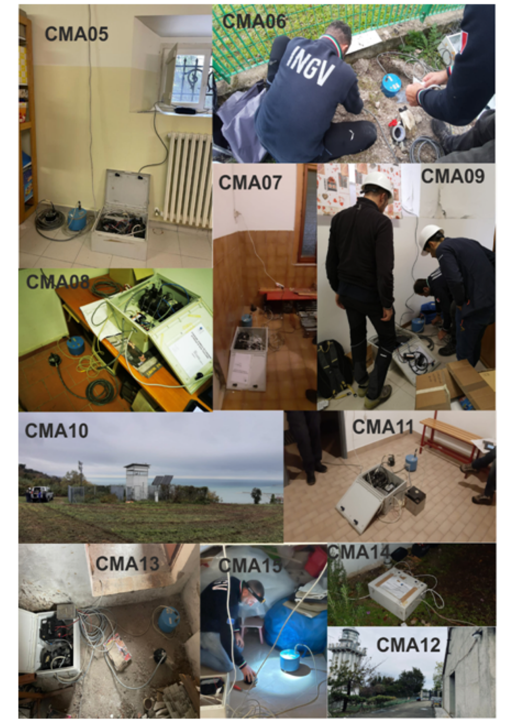
Figure 3.b Group activities and installations details: 11 stations equipped with Reftek130 + Lennartz 3D-5s velocimeter and Episensor accelerometer. Real time transmission to INGV data center.
