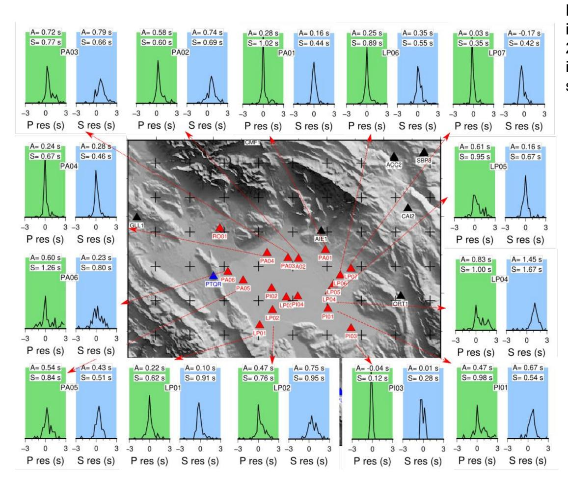
During the 2008-2009 time-window, 18 temporary seismic stations, operating in continuous mode at 125 Hz, were installed in the Fucino area to investigate the basin seismic response and local site effects (red triangles on the figures; Cara et al, 2011). This dataset was integrated by the permanent stations of the Italian seismic network and Abruzzo regional network installed on the surrounding ridges, to construct a new earthquake catalog and perform a local-scale passive tomographic survey.
