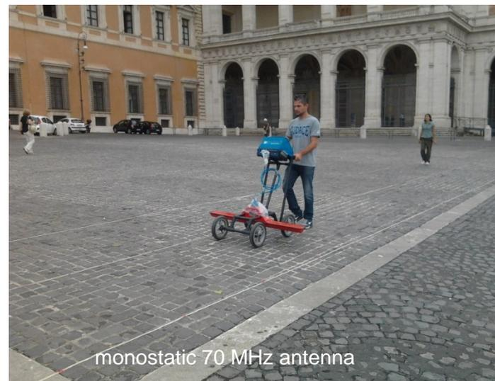
monostatic 70 MHz antenna
