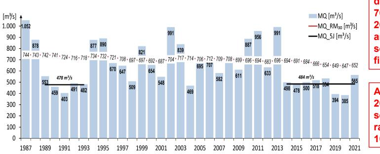
If the discharge drops from 700m<sup>3</sup>/s to 200m<sup>3</sup>/s, then the amount of sediments in HH is five times higher !
