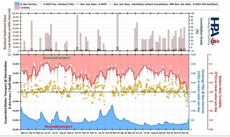
April 25th, 2023 - Monitoring of suspended mater with H-ADCP devices and comparison with sedimentation rates and soil properties in the Köhlfleethafen harbour basin of the Hamburg port - Nino Ohle - EGU 2023 -
