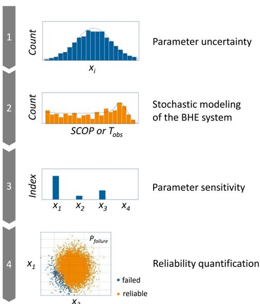
Figure 1 Main steps to quantify groundwater flow impacts on BHE system performance.
