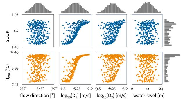
Figure 4 Simulated  $SCOP$  and  $T_{obs}$  versus stochastic groundwater flow parameters in the 10th simulation year.
