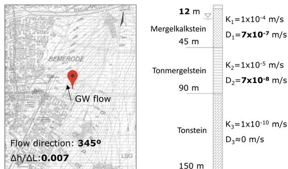
Figure 2 Hydrogeological map and typical borehole log at the Hannover site. Darcy flux in each layer is assumed.
