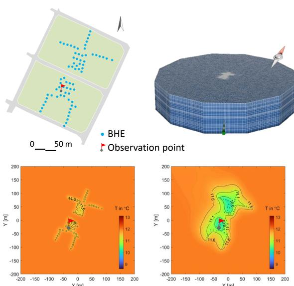
Figure 3 Arrangement of BHEs and 3D FEFLOW model (top), and simulated temperature maps in the 1st and 10th year for a parameter realization (bottom).
