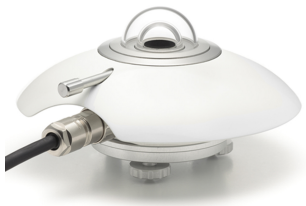
Figure: Pyranometer, used to measure Global Horizontal Irradiance (GHI), also known as SSR.
