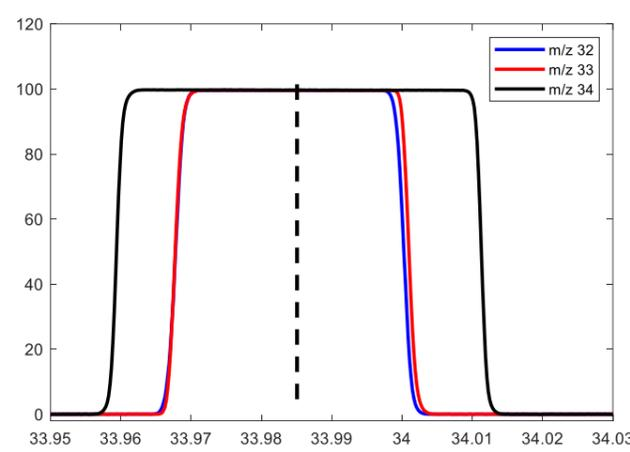
Figure 3: Overlaid mass scans of the  $O_2$  peaks at  $m/z$  32, 33 and 34. The dashed line indicates the measurement location (clumped traces not shown)
