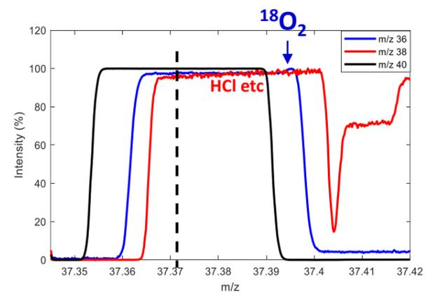
Figure 4: Overlaid mass scans of the  $Ar$  peaks at  $m/z$  36, 38 and 40. The dashed line indicates the measurement location - set on the left side of the  $m/z$  36 and 38 peaks in order to avoid some small interferences.
