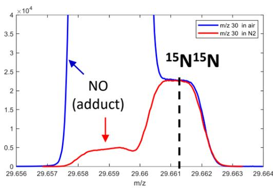
Figure 2: Mass scan around  $m/z$  30, showing the  $NO$  and  $^{15}N^{15}N$  peaks. The dashed line indicates the measurement location.
