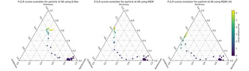
**Figure 8.** The texture of this particle is represented by pointiness, girdleness, randomness scores that are calculated from the eigenvalues of the orientations.
