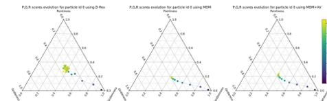
**Figure 4.** The texture of this particle is represented by pointiness, girdleness, randomness scores that are calculated from the eigenvalues of the orientations.
