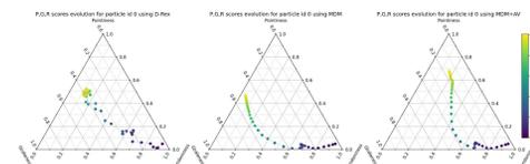
**Figure 12.** The texture of this particle is represented by pointiness, girdleness, randomness scores that are calculated from the eigenvalues of the orientations.
