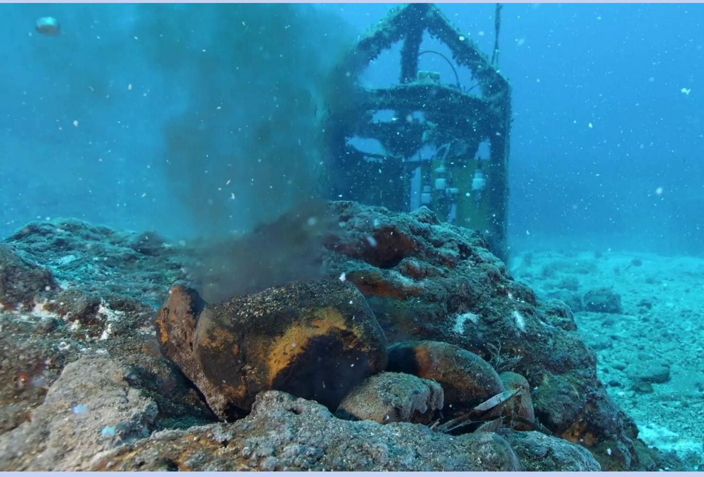
seafloor observatory installed close to the "Black Point" vent. This fixed connected by an umbilical cable to a surface buoy, which provides power to the whole system by solar panels and a battery pack.
