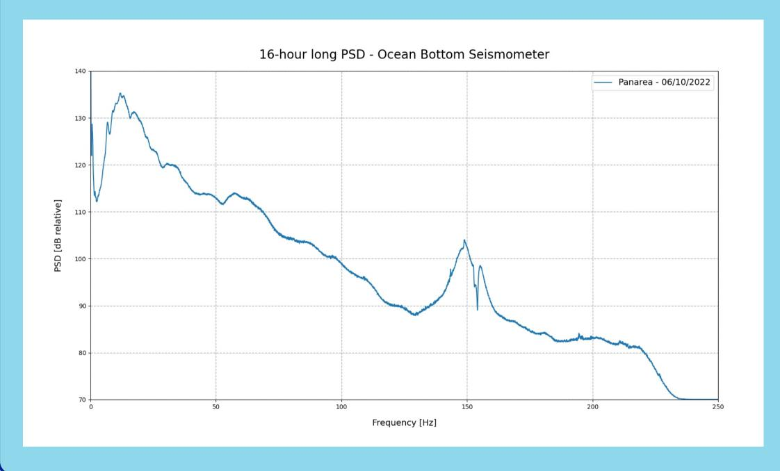
The deployment of an OBS in October 2022 further confirmed the mechanisms behind the fluid dynamics. Narrow peaks (~25 Hz and ~150 Hz) highlight the resonance of the conduit crossed by ascending turbulent flow.
