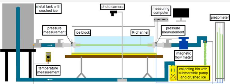
Fig. 1: Sketch of the set up of the laboratory experiment
