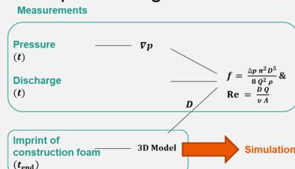
Fig. 3: Visualization of the data flow. Upper green frame emphasizes the analysis of the laboratory experiment while the lower one is framing the process leading to the numerical simulation.
