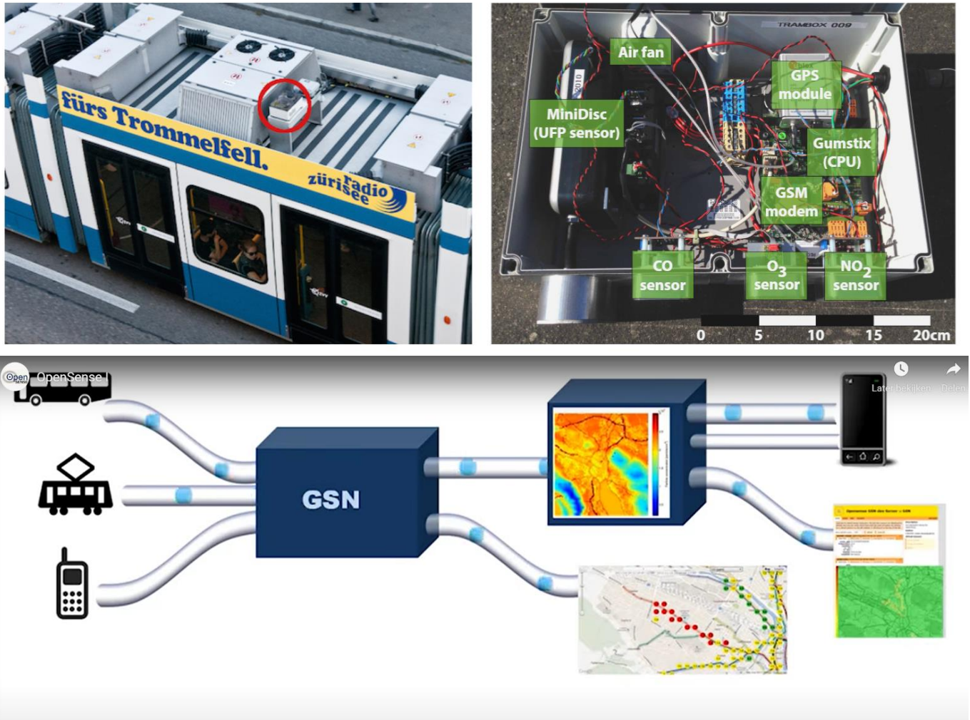
Figure 16: The Opensense sensor node (upper; from Hasenfratz et al., 2015) and data pipeline (lower) with mobile air quality data collected by the Global Sensor Networks (GSN), visualisation dashboard of the measurements and trained spatiotemporal model and visualisation.
