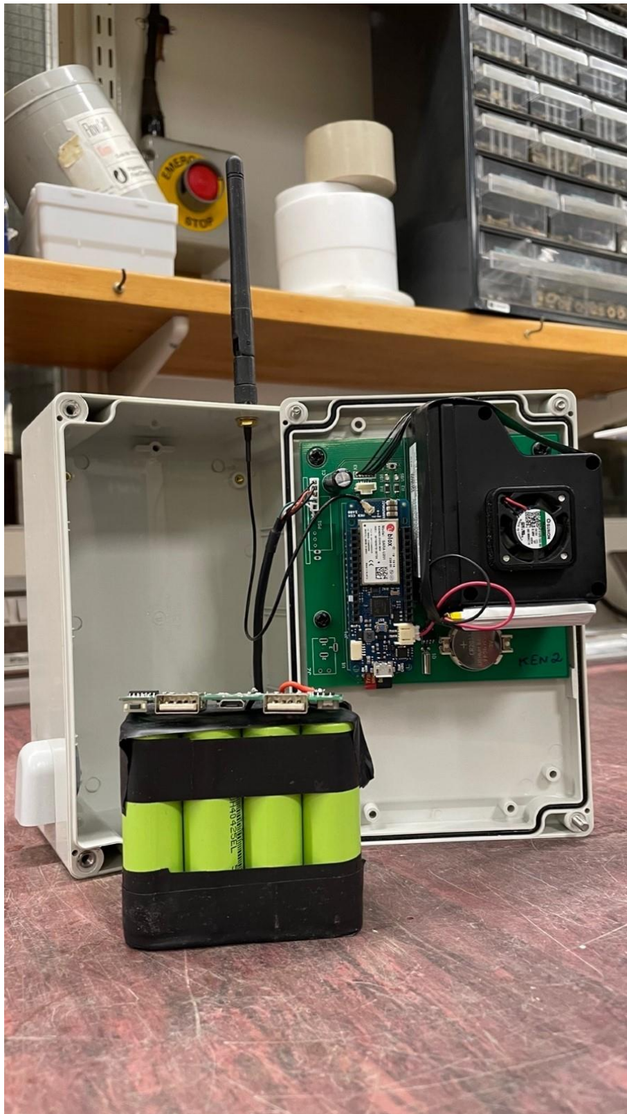
Figure 27: An opened case of the mobile measurement setup. The current iteration can collect and upload to the cloud PNSD, PM mass measurements, and geolocalisation data for about 2.5 days. Weighs about 500 grams with the battery installed.
