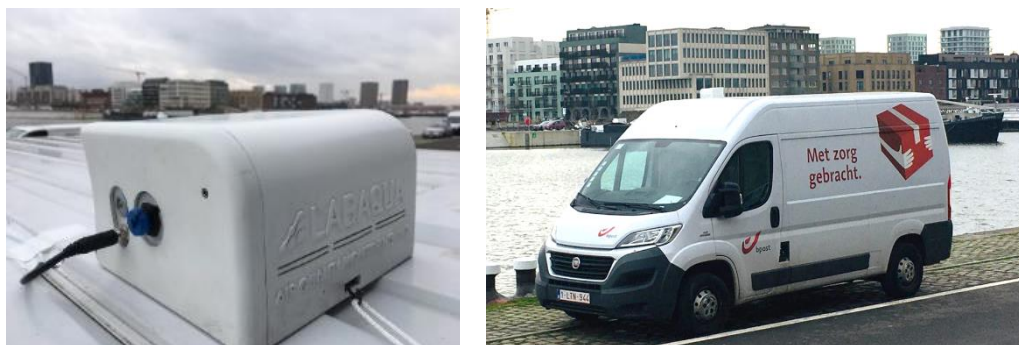
Figure 7: Kunak Air Mobile sensor unit in its dedicated LABAQUA housing, deployed on the roof of a postal van.
