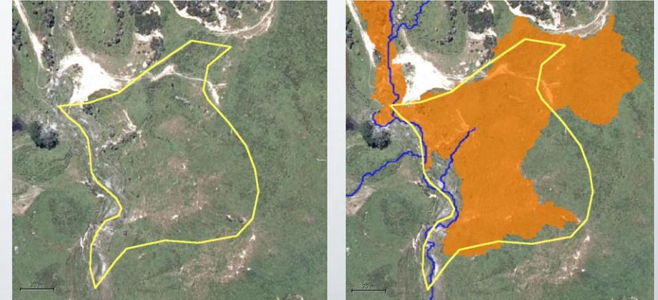
Earthflow mapping examples. OBIA mapping (orange) in comparison to reference data (yellow outline). Channel network is shown as blue lines.
