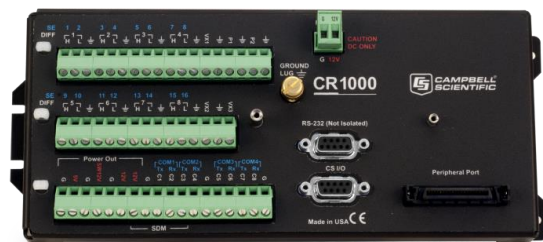
Figure 2. The Campbell Scientific CR1000 datalogger uses TTL to send requests for and receive data from our tilt sensor system.
