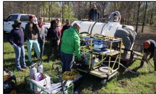
Figure 1: from left to right: A visual representation of the new technique utilized extracting water and cycling the water with chlorine gas infused bleach production on demand in the field with a mobile cart; The current oxalic acid trailer treatment system next to the relief well drainage ditch parallel to the levee at Eagle Lake Levee and Tara Wildlife Area, MS, the photo also shows the RWS system that is planned to be incorporated on a trailer treatment system; The top of the relief well at the levee (the well is 90 ft in depth); and an ERDC scientist and engineer collecting water samples to investigate the biofilm presence before and after treatment.
