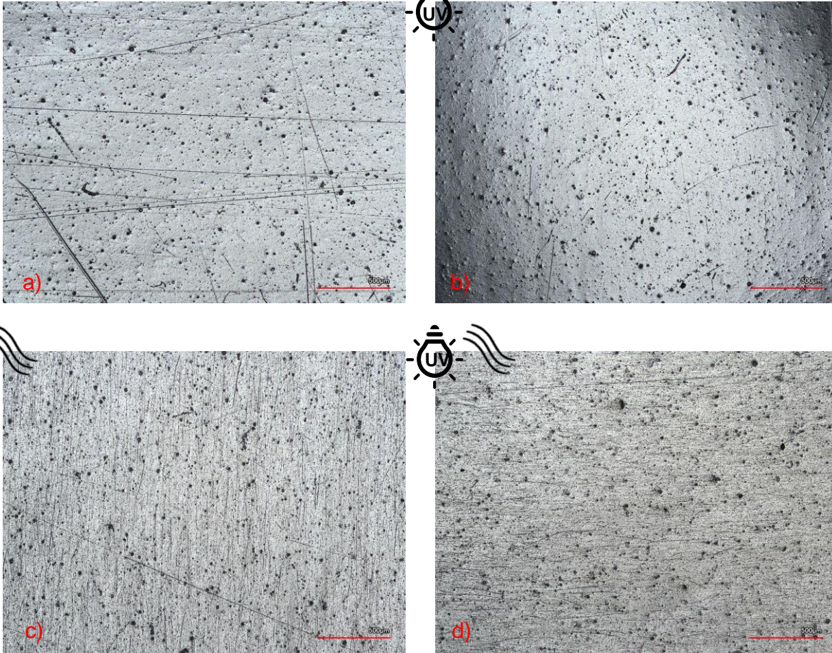
Figure 11: Laser scanning microscope images, 500 μm. a) and b) Black and white 1, white part (100 μm), 0 and 80 days UV degraded, respectively; c) and d) Black and white 1, white part, 0 and 80 days UV degraded combined with abrasion, respectively.
