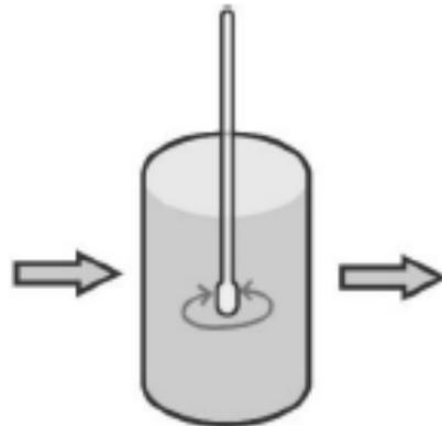
$$\frac{d(C.V)}{dt} = Q_{in} \times C_{in} - Q_{out} \times C_{out} + r_p \times V - r_c \times V$$
