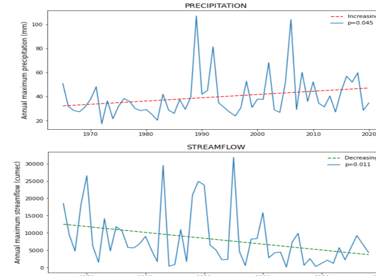
Fig. 3. Observed annual maximum precipitation and streamflow at the Mancherial stream gauging station
