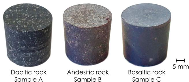
Fig. 1. Three types of volcanic rocks used in the chelating agent flooding experiments: Sample A, Sample B, and Sample C were prepared from dacitic, andesitic, and basaltic rocks, respectively.
