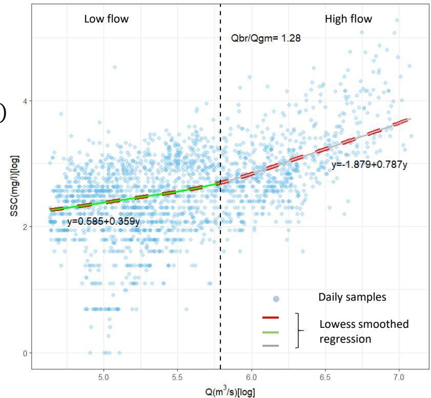
=> I opted for rating exponent extracted at high flows using NLS since it can catch high values of pairs (SSC, Q) and gives more significant slopes although  $R^2$  is not always the highest
