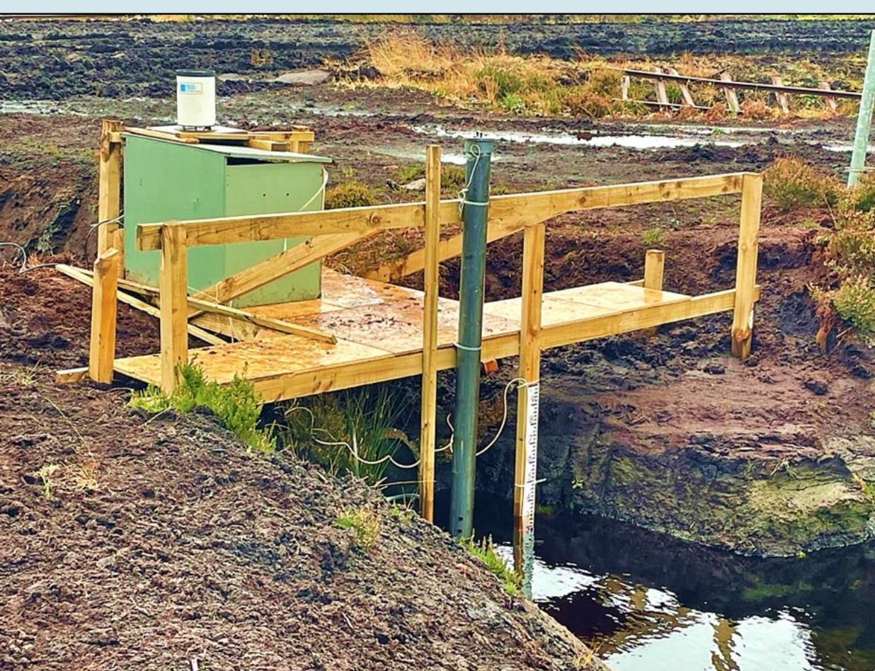
Fig. 2. Monitoring station of water quality at the outlet of the treatment pond.
