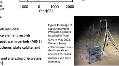
Figure 11: Image of Syp autosampler (Waikato Scientific) installed in Titan Cave in May 2022. Water is being collected over four-day intervals and analyzed for stable isotopes and trace elements.
