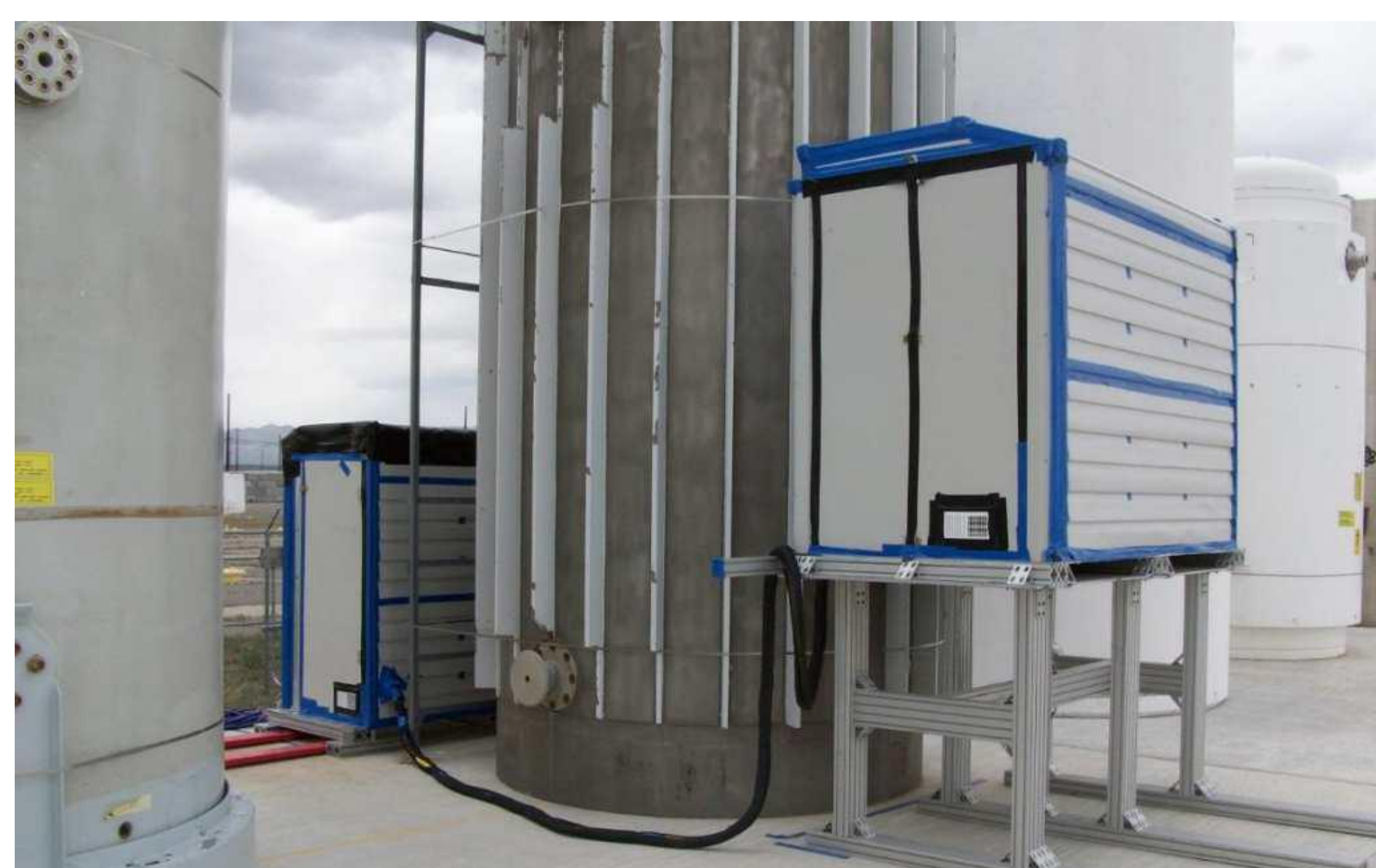
Muon tracking supermodules placed on opposite sides of the Westinghouse MC-10 Fuel Cask at Idaho National Laboratory.
