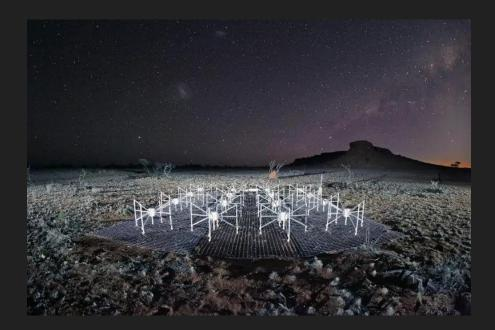
Murchison Widefield Array (MWA) (Square Kilometre Array precursor) 128 (currently 144) antenna tiles, 80 - 300 MHz, 30.72 MHz bandwidth, 10 kHz, 0.25 s (Tingay et al. 2013, Wayth et al. 2018)
