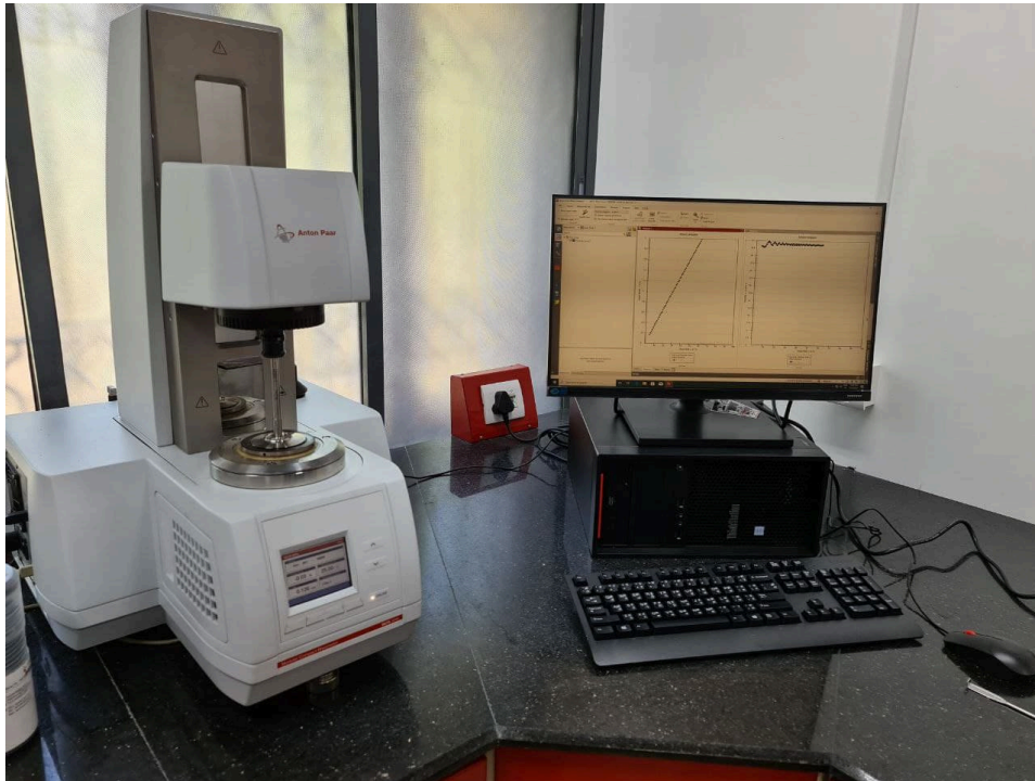
73 Figure S1. Laboratory setup (Anton Paar Modular Compact Rheometer 302e) used for the 74 rheological tests of experimental model materials.
