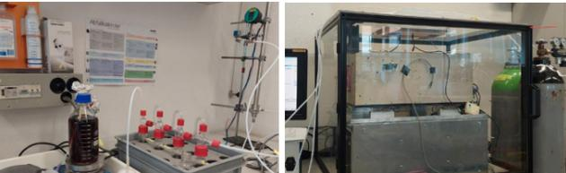
Fig. 1 – Pictures of the current setup: bacteria culture with an alkaline CO<sub>2</sub> trap and a permeation dryer (left); QCLAS with mass flow controllers (MFC) (right).
