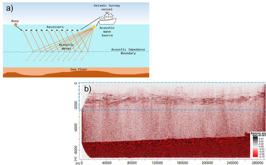
Figure 1: a) Multichannel Seismic acquisition diagram; b) Final stacked image of the ocean acquired 2D line.
