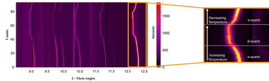
We performed a sequential refinement to obtain **volume** and **cell parameters**. At the same time, we collected **wave velocities** from double travel times and X-ray absorption images of the sample.
