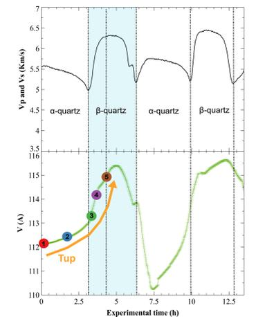
At this point, one can calculate the elastic moduli from  $V_p$  and  $V_s$ . In our results, we obtain that the bulk modulus (K), calculated at a constant pressure of 1 GPa and during a temperature ramp, has values of around 30 GPa in the  $\alpha$ -field and of around 55 GPa in the  $\beta$ -field. Interestingly, the bulk modulus does not drop to 0 GPa at the transition and is significantly weaker than predicted by the EoS calculations.
