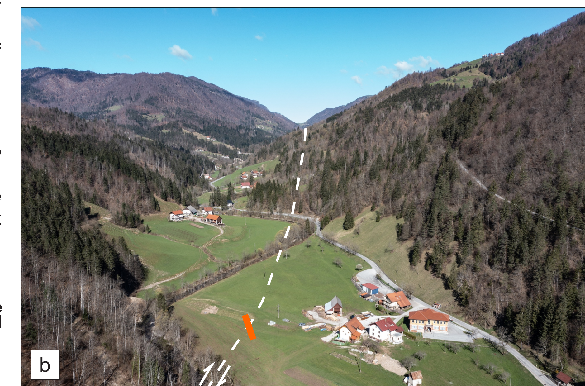
Figure 4: a) Highly expressed morphology of the seismically active Idrija fault. b) Position of „Hall effect“ creepmeter across the Idrija fault.
