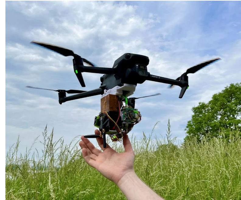
Figure 9: Picture of little-RAVEN during a handheld take-off. Under the drone, the adapter plate and the sensor system can be seen.
