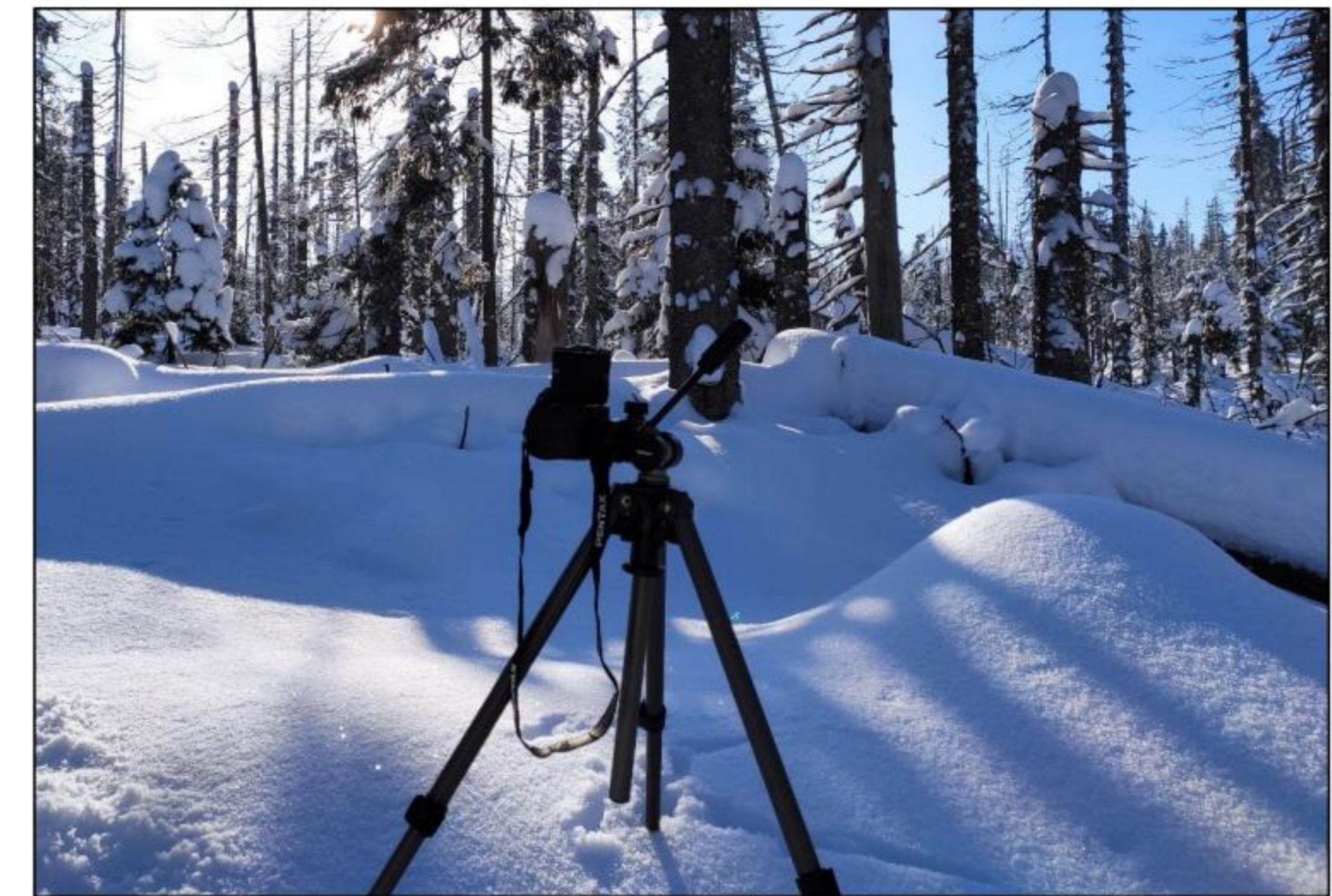
Capturing hemispherical images with a Pentax K-5 IIs digital mirror camera with fisheye lens
