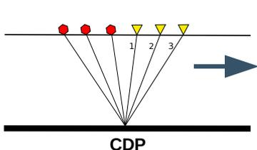
1. Source-receiver combinations for which the points of reflection fall into pre-defined bins are selected.
