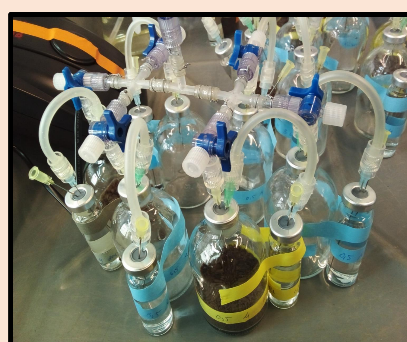
Figure 3: Mesocosm setup with main soil chamber and connected CO 2 traps [3]
