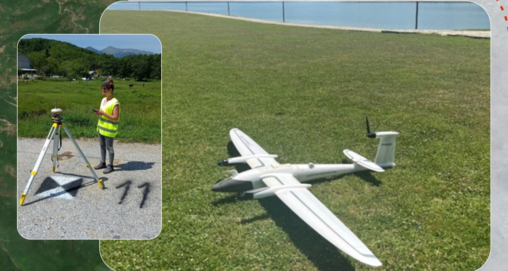
The equipment for the onshore data collection included a fixed wing UAS (upper inset), which covered the entire coastal area, acquiring thousands of aerial images used for constructing high-resolution DTMs and ortho-mosaics (inset below). Also, GCPs were established around the lake with GNSS used either for post-processing of the aerial data and for combining the offshore data as well.
