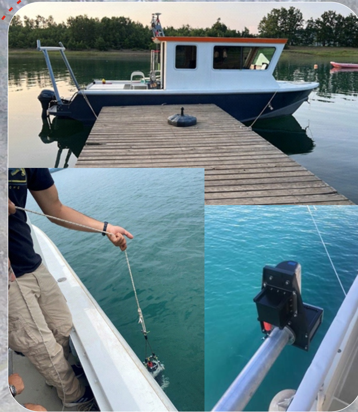
The equipment for the offshore, lake bottom data collection, included a multi-beam sounding device carried by a vessel, conducting transects parallel to the main lake axis (right inset).
