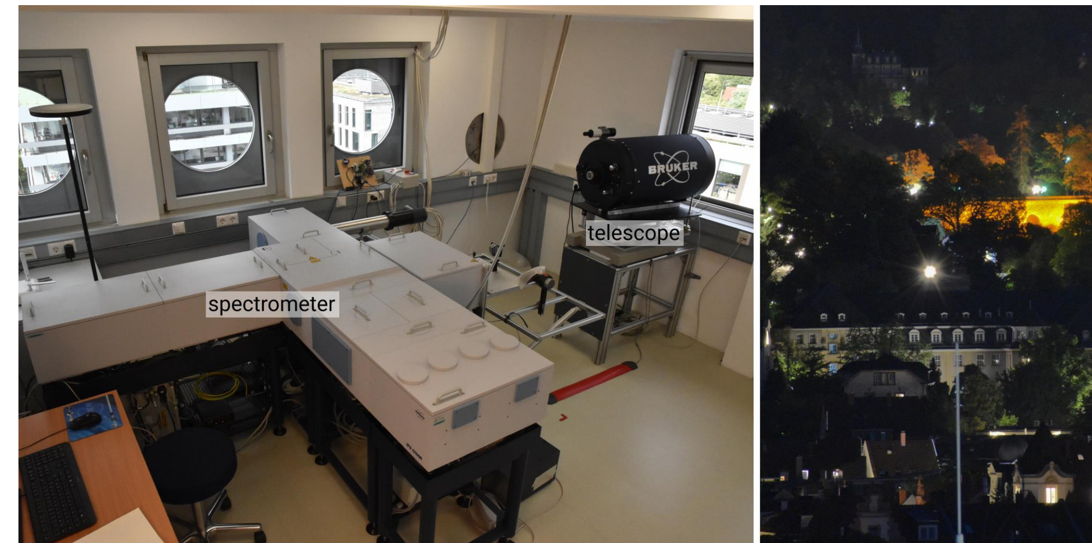
Left: Fourier Transform Spectrometer and the telescope for the open-path setup. Right: Reflector at the eastern end of the path at night.
