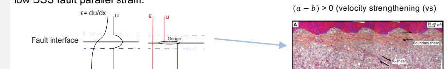
Figure 8. Schematics of the effect of gouge on the strain and slip during the subsequent steps of the experiment.
