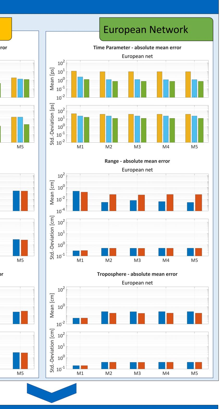
Equal weighting **improves** parameter **estimation** significantly Time parameters can be estimated with picosecond precision and accuracy Stronger weight on optical "true" range observations brings benefit
