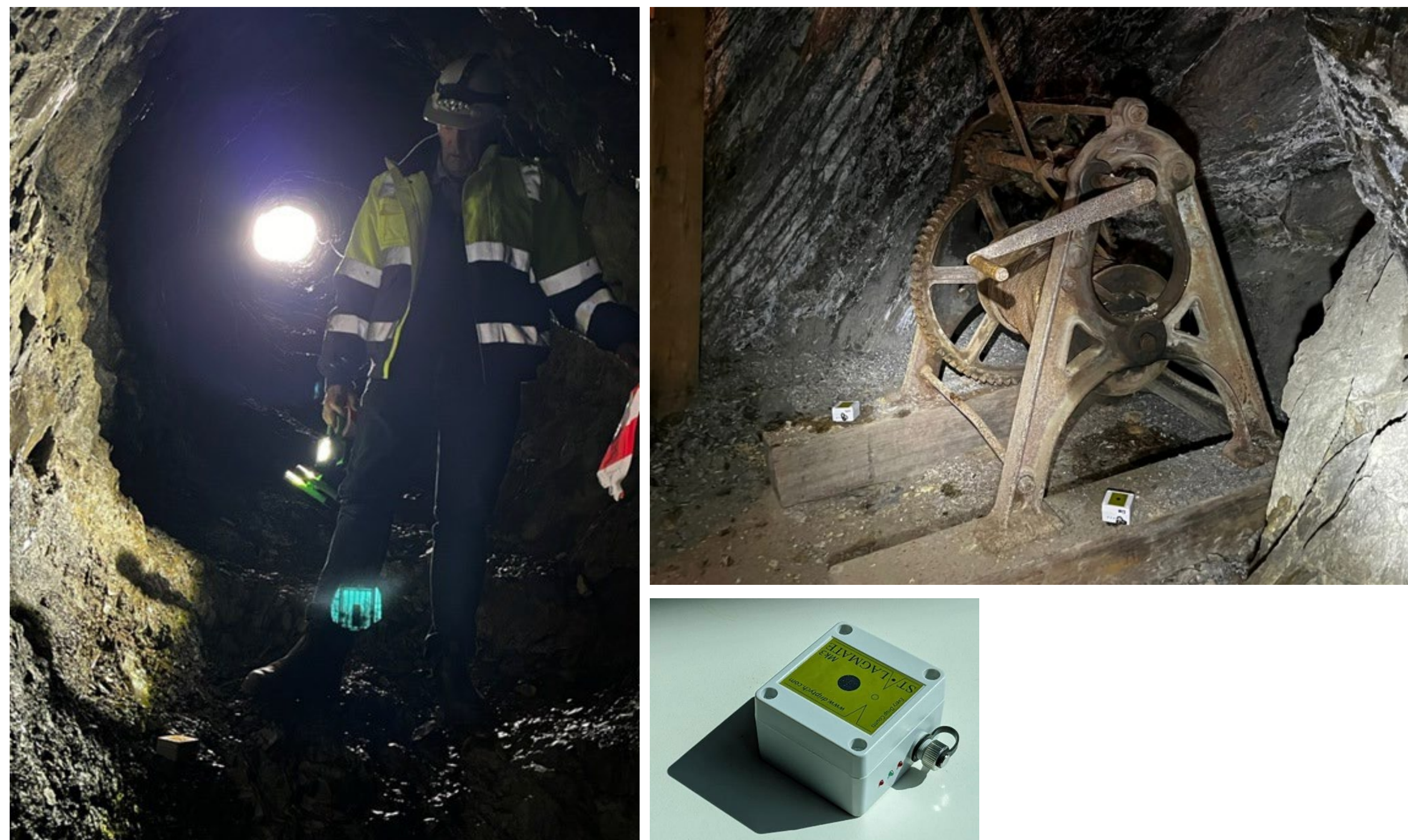
Fig. 3. Photos of Walhalla gold mine emergency exit tunnel with drip sensors at regular intervals & overburden depth from <10 m to >70 m. The sensors (INSET) are on the floor recording water dripping from the mine roof.
