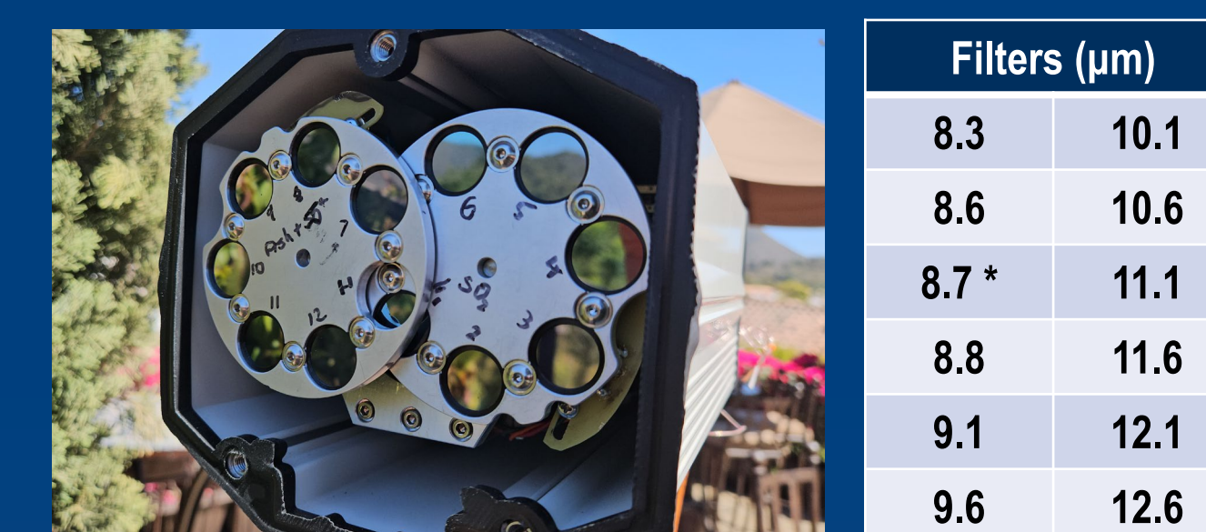
Figure 17. MMT-gasCam filter wheels shown with germanium cover window removed. The filter wavelength centers are shown in the table. *broadband (1.0 μm) SO 2 filter.
