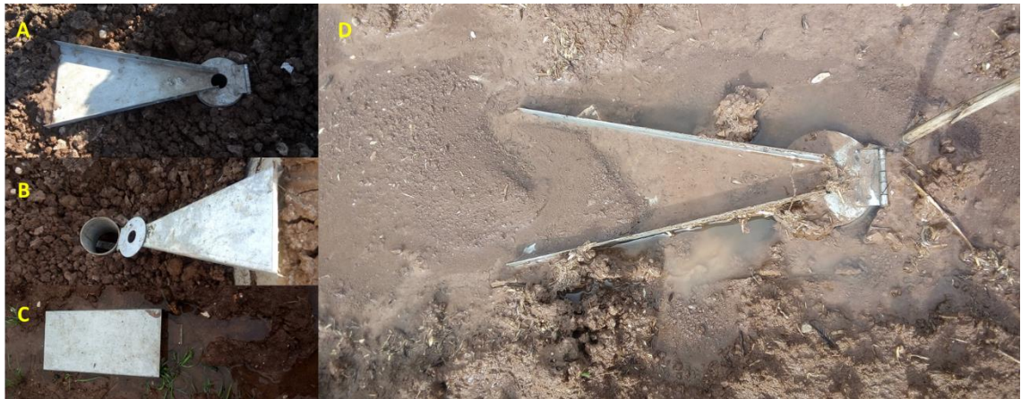
Figure 3S: RCU (A) installed before rain; (B) RCU with flume open. The glass bottle is inserted into the designated cylindrical space; (C) Ready for the storm, RCU with the roof protecting rain dilution; and (D) RCU after removing the roof to collect the full sample.
