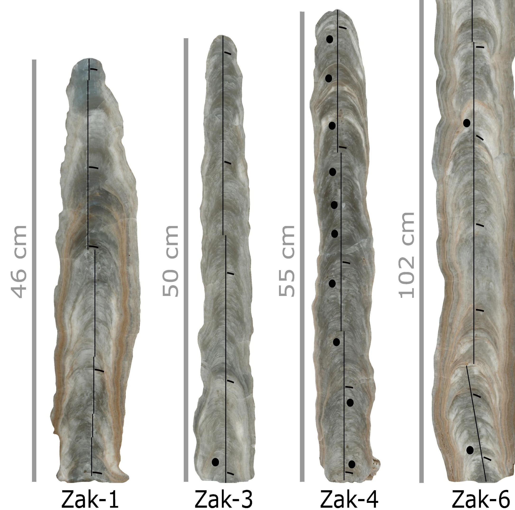
Fig. 2. Zak speleothems. Vertical lines identify the stable isotopes track. Horizontal bars point to the stratigraphic locations of U-Th subsampling. Circles indicate location for fluid inclusions subsampling.
