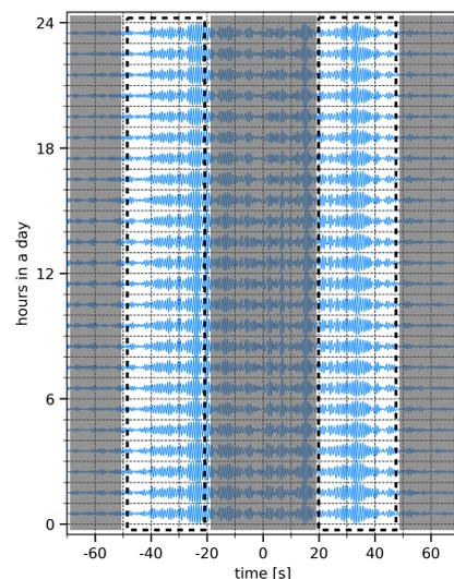
Fig. 2 Stacked cross-correlation for every hour for a station pair in northern Italy. Each trace represents the stack of all corresponding hour within the time period. The highlighted part represent the coda wave window.
