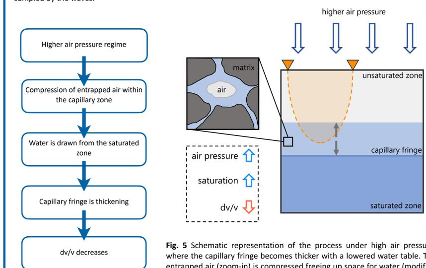
Fig. 5 Schematic representation of the process under high air pressure, where the capillary fringe becomes thicker with a lowered water table. The entrapped air (zoom-in) is compressed freeing up space for water (modified after Fabbri et al. 2019). The orange shaded area is a simplistic represent the parts sampled by the waves.
