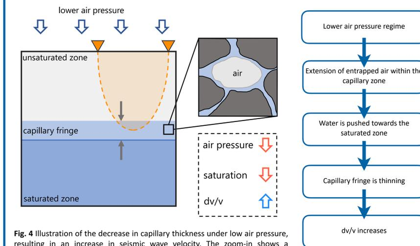
Fig. 4 Illustration of the decrease in capillary thickness under low air pressure, resulting in an increase in seismic wave velocity. The zoom-in shows a representation of entrapped air in a low pressure regime (modified after Fabbri et al. 2019). The orange shaded area is a simplistic represent the parts sampled by the waves.
