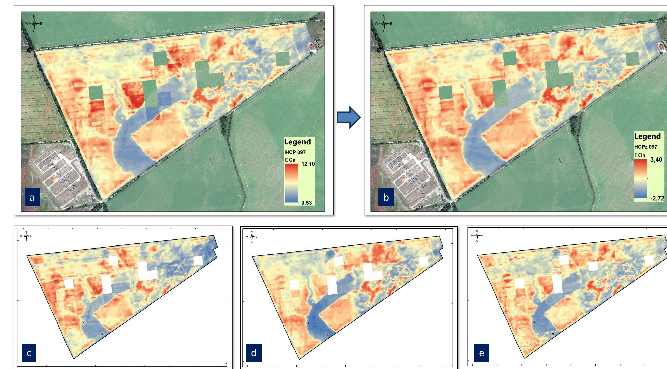
a) Filtered ECa map (HCP mode coil-3 with DOI up to 108 cm), b) ECa map after Z-transformation normalization. This highlights the intra-field variability and removes the influence of temporal changes in environmental conditions. c) Normalized ECa map of HCP 0-52 cm, d) HCP 0-270 cm, e) VCP 0-118 cm
