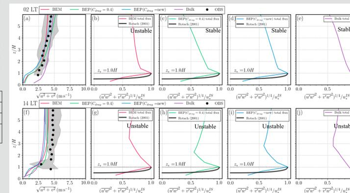
Figure 6: Wind speed and Reynolds stress profiles averaged at 02 (night) and 14 (day) local time (LT). The y-axis is normalized by the building height which is homogeneously 60 m. The black markers represent the LiDAR observations for wind speeds, and the black solid lines depict the  $u_*$  calculated from Eqn. 2
