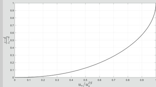
Figure 1: Local friction velocity  $u_*$  as a function of non-dimensional height. Reproduced from Rotach (2001) following Eqn.2
