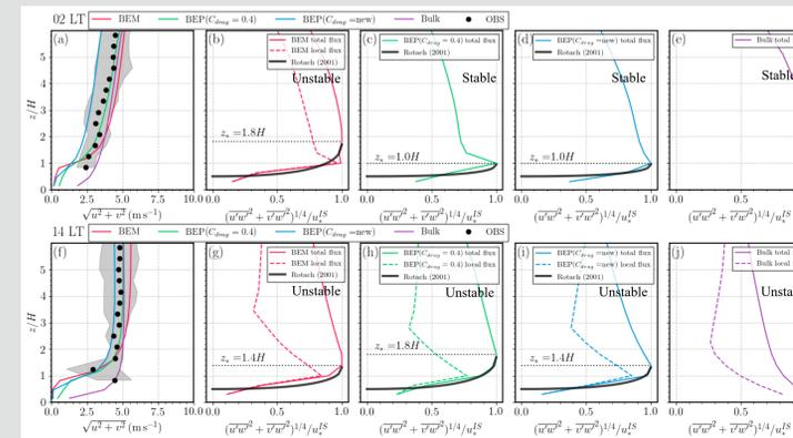
Figure 4: Wind speed and Reynolds stress profiles averaged at 02 (night) and 14 (day) local time (LT). The y-axis is normalized by the building height which is homogeneously 60 m. The dashed lines represent the local fluxes ( $-K \frac{\partial u}{\partial z}$ ). The black markers represent the LiDAR observations for wind speeds, and the black solid lines depict the  $u_*$  calculated from Eqn. 2
