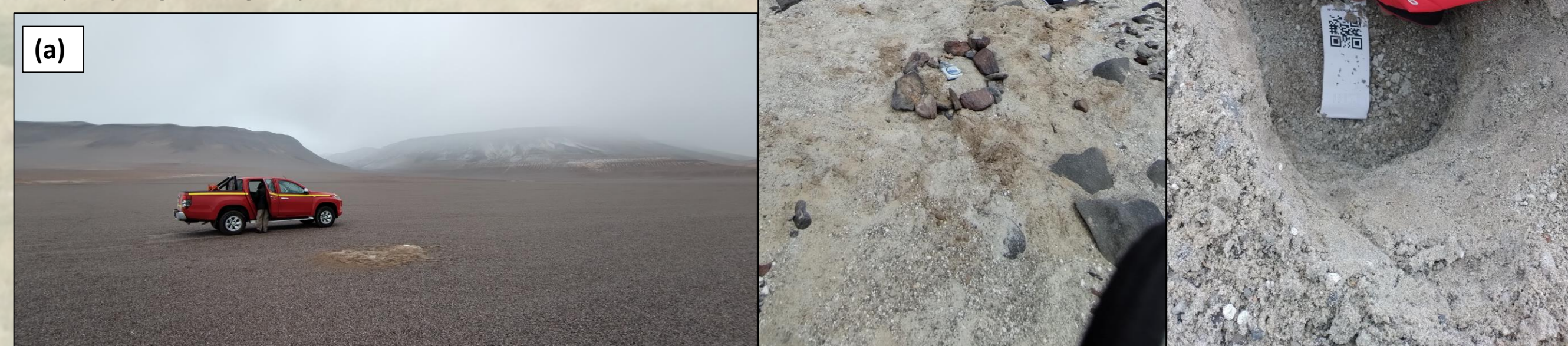
Figure 3: (a) Station installation near Laguna Verde, (b) a high altitude station is marked with rocks for visibility and to shield cables from the wind, (c) measuring permafrost depth at one high altitude station site before deploying the geophone in the hole.
