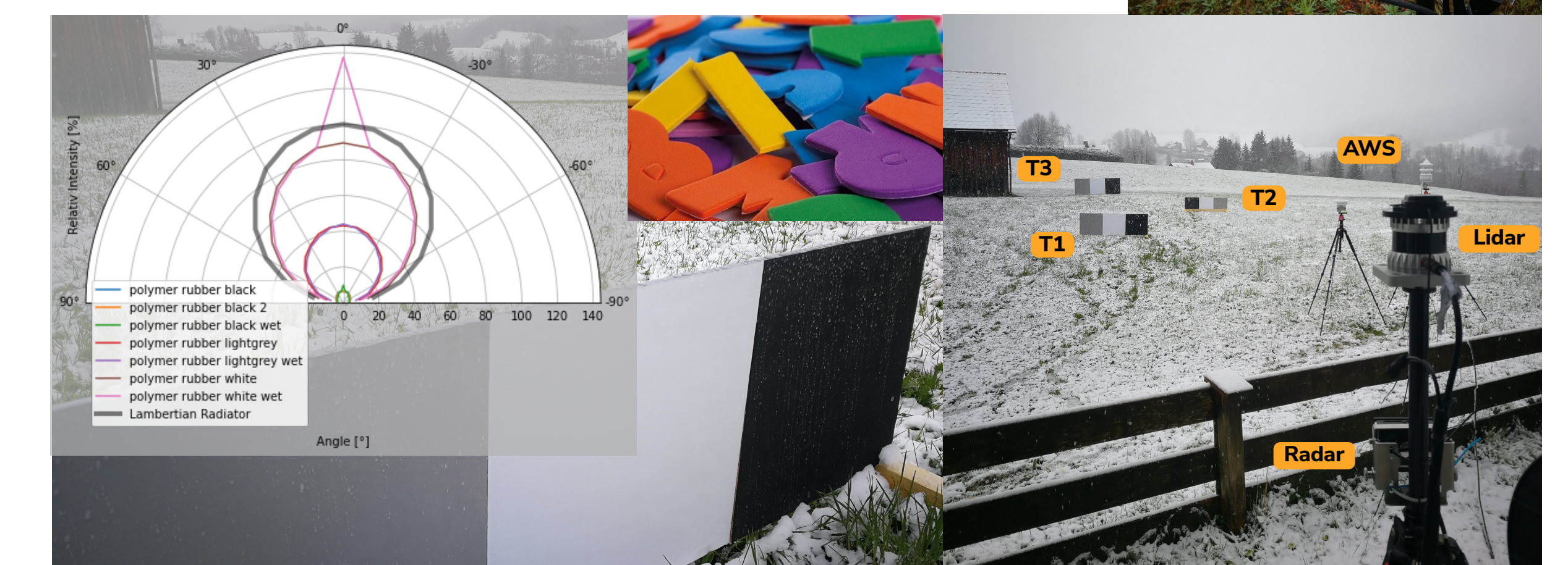
D Top: Long term measurements of liquid precipitation at roof top with five targets. Bottom left: Foam rubber as lambertian targets. Bottom right: Measurement campaign with lidar and radar in snowfall and three targets (T1-T3) at various distances.
