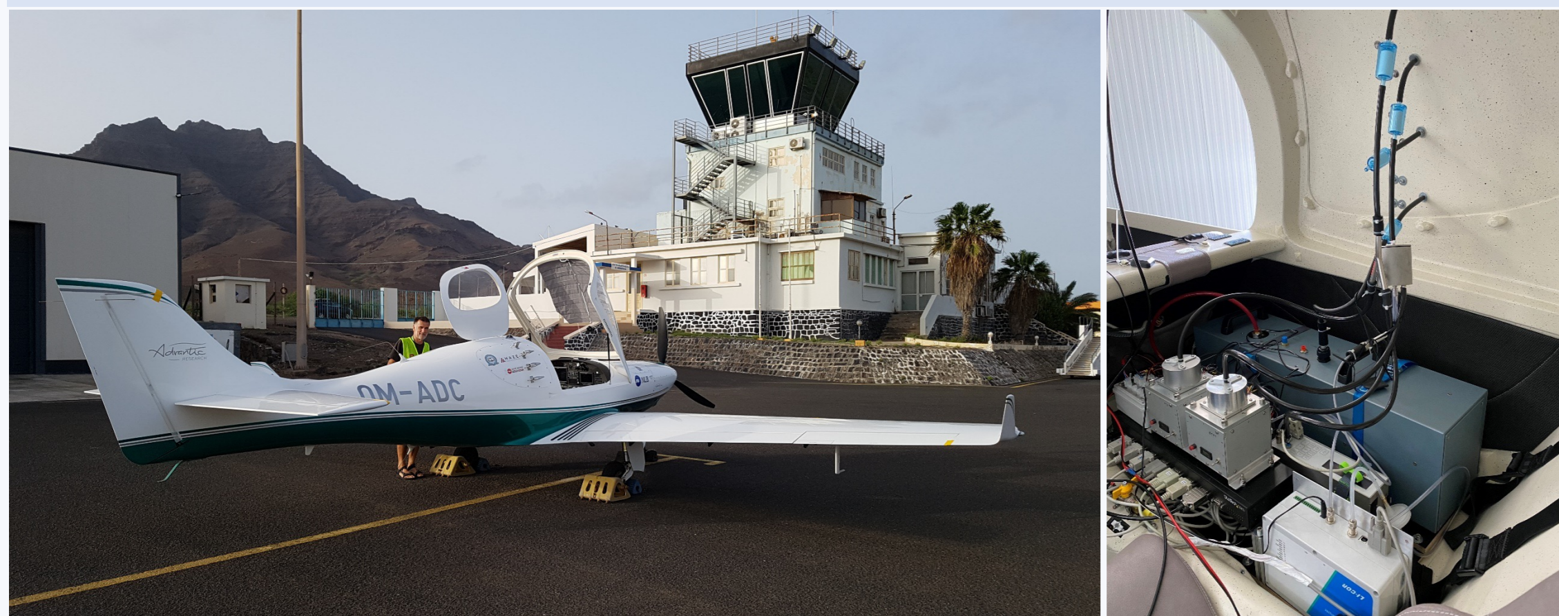
[Left] Ultralight airplane Aerospool Advantic WT-10 equipped with inlets for fine and coarse aerosols and [Right] two Continuous Light Absorption Photometers for aerosol light absorption measurements at the fine and coarse fraction, a polar integrating nephelometer Ecotech Aurora 4000 for aerosol light scattering measurements, two optical particle counters for measuring the particle size distribution and additional meteorological sensors (CO2 sensor, RH).
